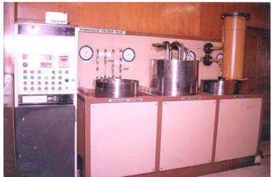
Filter test rig
